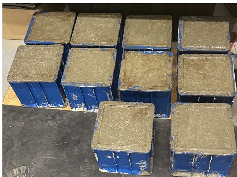
Figure 1. Concrete cube specimens (15 cm × 15 cm × 15 cm) after casting in steel molds. The molds were filled in three layers, each compacted with 35 blows, following ASTM C192.
