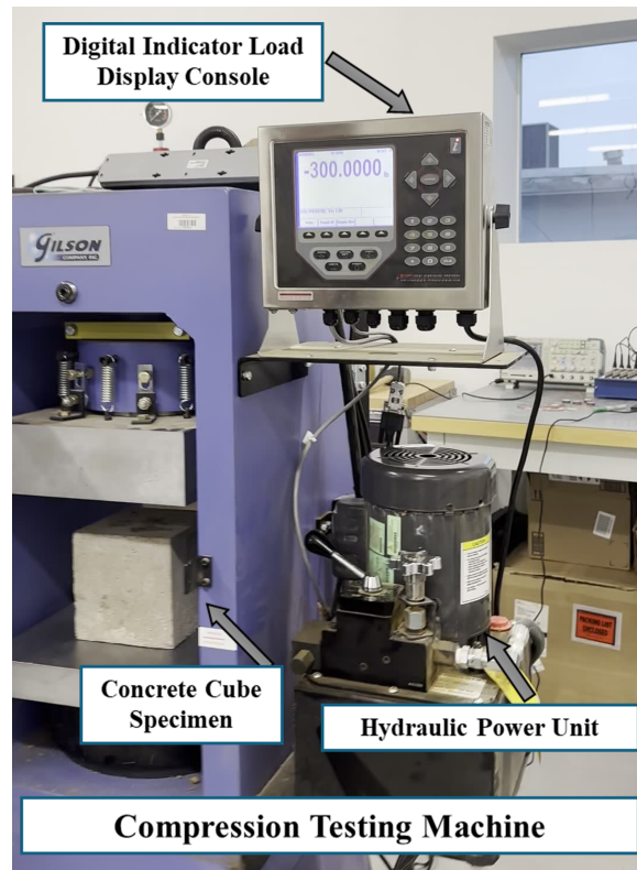
Figure 3. Labeled components of a compression testing machine (Gilson Company, Lewis Center, OH, USA) used for evaluating the compressive strength of concrete specimens. The setup includes a concrete cube specimen placed between loading platens, a Digital Indicator Load Display Console for monitoring applied load, and a Hydraulic Power Unit that drives the loading mechanism.
